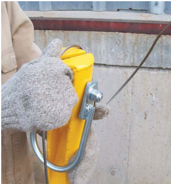
Figure #5.2f: Inserting the winch cable into the offset arm's pulley slot
