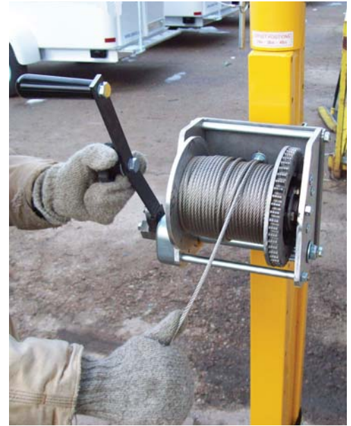
Figure #5.2d: Retrieval winch mounted at the rear of the centerpost
