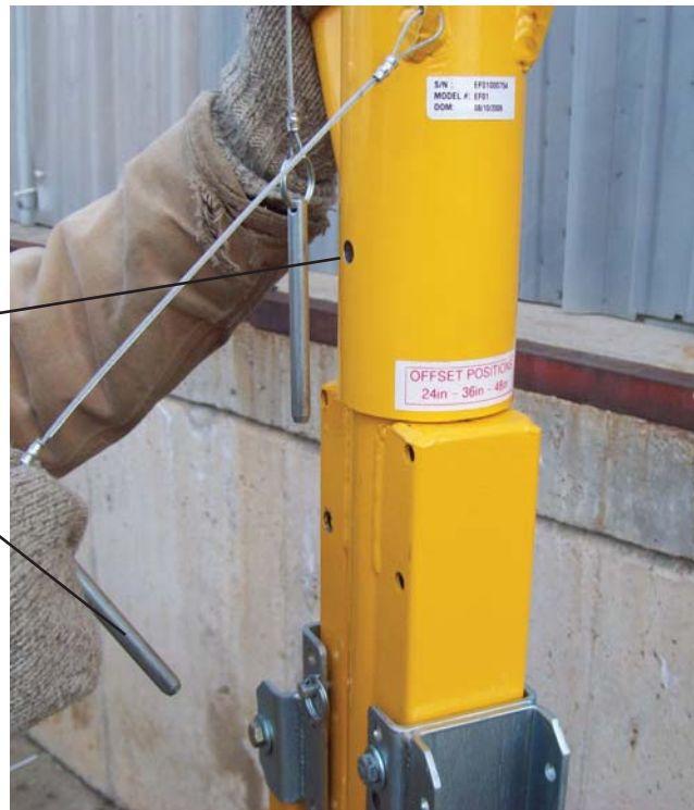
Figure #5.2c: Securing the elbow to the centerpost
