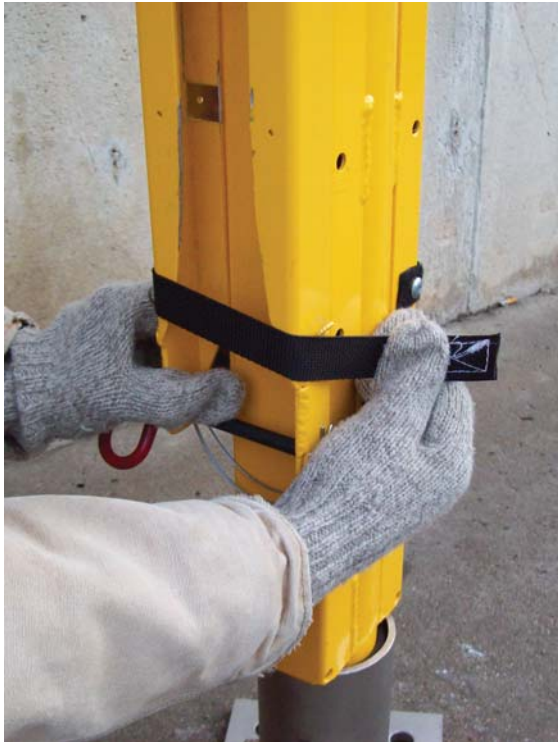
Figure #5.2h: Elbow support frame securing strap
