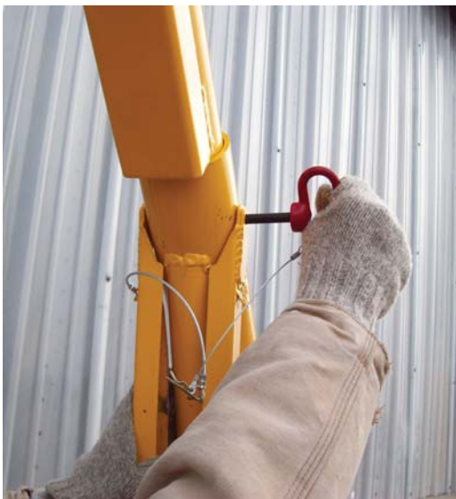
Figure #5.2j: Pinning the offset arm, elbow & elbow support frame.
